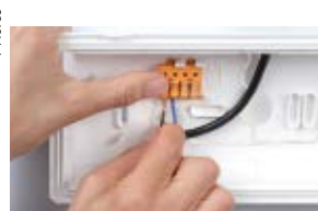
The body can be pre-installed. Just insert the cable through the cable gland, insert the wires into the screwless connector and just click the reflector into place.
