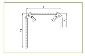
Your solution: ERJ-A<sup>1</sup>LA Min. A<sup>1</sup> = 250 mm Max. A<sup>1</sup> = 1000 mm Min. L = 380 mm Max. L = 1000 mm Min. A = 250 mm Max. A = 1000 mm
