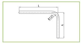
Your solution: ERL-LA Min. L = 250 mm Max. L = 1000 mm Min. A = 250 mm
